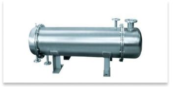
Shell and tube heat exchangers are considered one among the most effective type of heat exchangers. These heat exchanges have a cylindrical shell with a bundle of tubes. The tubes are made from thermally conductive materials, which allow heat exchange between the hot fluids flowing outside the tubes and the coolant flowing through the tubes.
